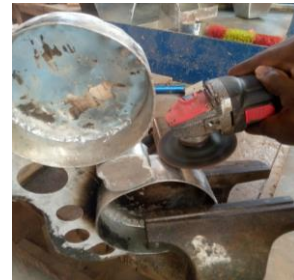
Figure 49. Grinding of the Saanbu symbol
