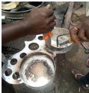
Figure 38. Welding the various parts of the Saanbu symbol
