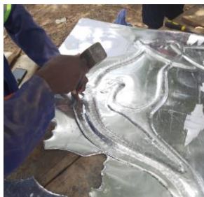
Figure 32. Cutting out the embossed Daŋ-taa symbol from the parent material
