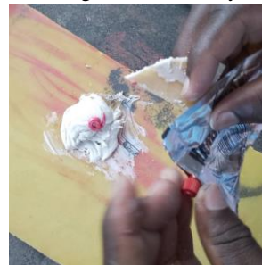
Figure 51. Mixture of the filler
