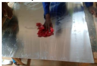
Figure 24. Preparation of the aluminum metal plate
