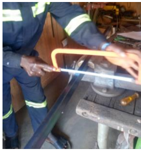
Figure 42. Cutting the marked parts of the frame
