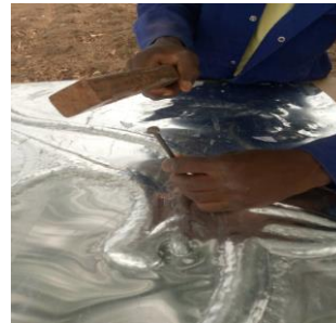
Figure 29. Chasing around the embossed areas
