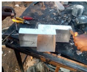
Figure 36. Soldering to connect the various parts of the central container
