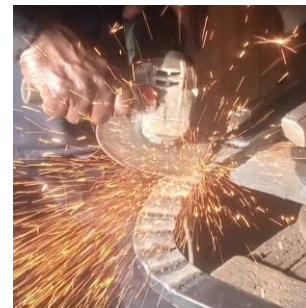
Figure 47. Sanding the curved part of the frame
