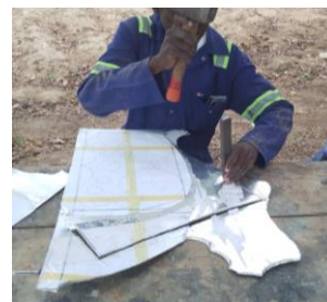
Figure 33. Cutting of the cup-like parts
