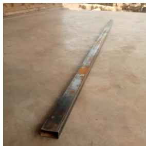
Figure 40. 1' x 2'' metal square pipe for the frame
