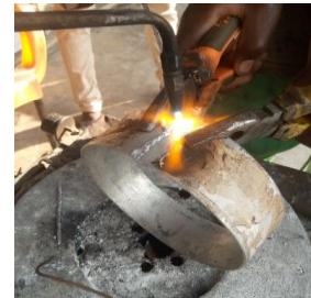
Figure 37. Soldering the joint of the circular parts of the Saanbu symbol
