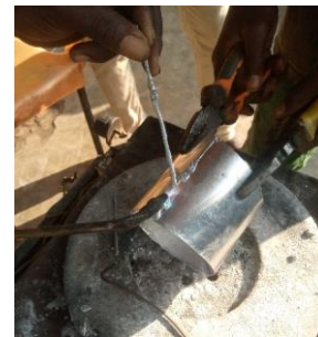
Figure 39. Soldering the back of the cup-like container
