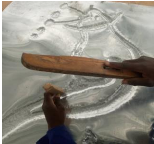
Figure 28. Embossing the design on the metal surface
