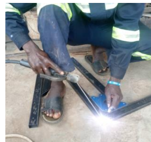
Figure 44. Using a magnetic tool to hold the angles of the frame accurately for welding
