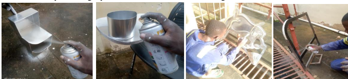
Figure 54. Spraying and drying of components
