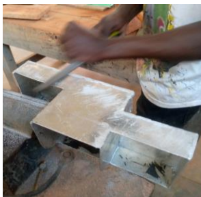
Figure 50. Filing to ensure a smooth surface
