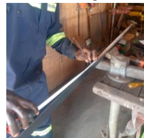
Figure 41. Measuring and marking areas to be cut
