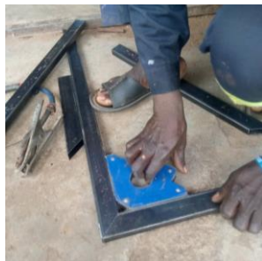
Figure 44. Using a magnetic tool to hold the angles of the frame accurately for welding
