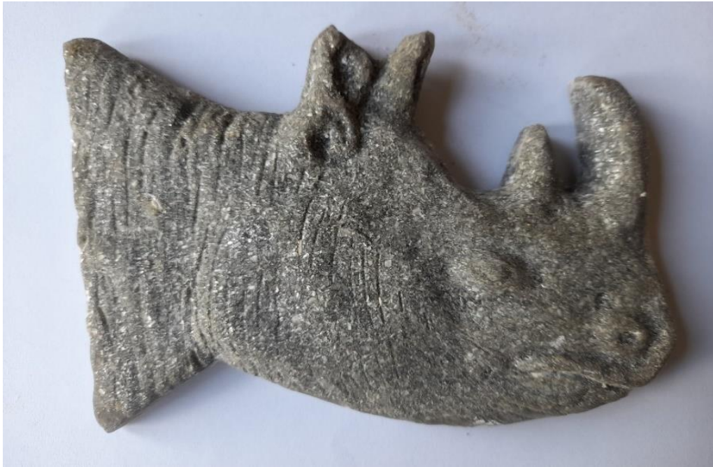
Figure 4.2 Final Cast of Head of a Rhinoceros from Solid Waste Aluminium Chips Source: Field Study, 2022
