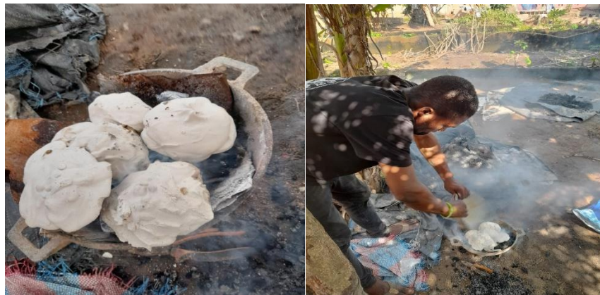
Figure 3.47(a and b) Students Dewaxing Source: Field Study, 2022
