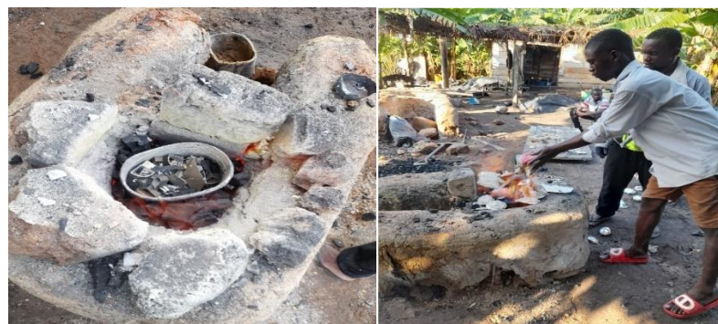
Figure 3.48 (a and b) Students Melting the Solid Waste Aluminium Source (Field Study, 2022)
