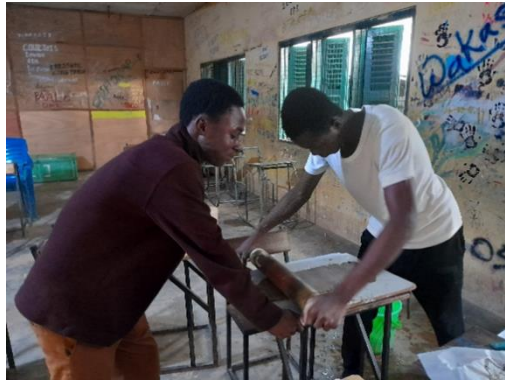
Figure 3. 32 Making Wax into Sheets
