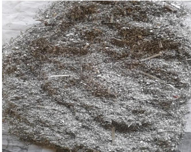
Figure 3.10(b) Aluminium Chips from Aluminium Window and Door Frame Manufacturers
