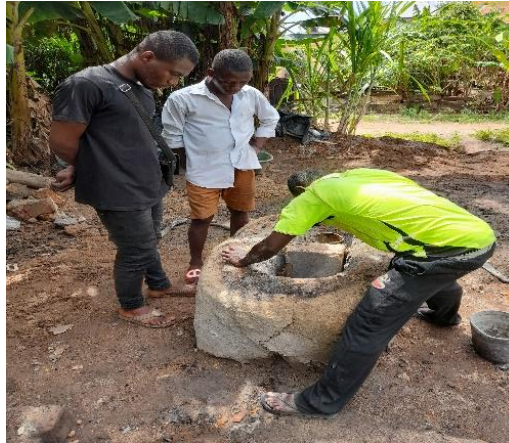
Figure 3.46 Preparing the Fire Furnace Source: Field Study, 2022
