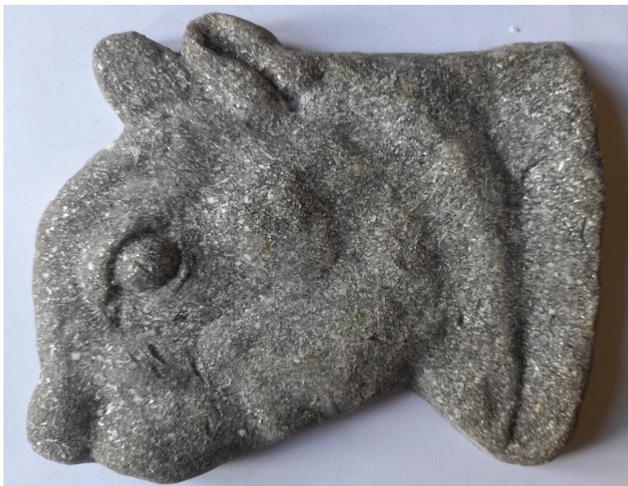
Figure 4.3 Final Cast of Head of a Rat from Solid Waste Aluminium Chips Source: Field Study, 2022
