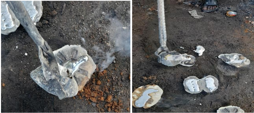
Figure 3.49 (a and b) Pouring the Molten Metal into Plaster Mould
