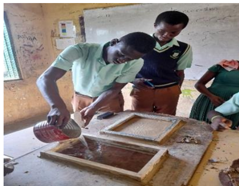
Figure 3.31 Pouring Wax into Wooden Mould
