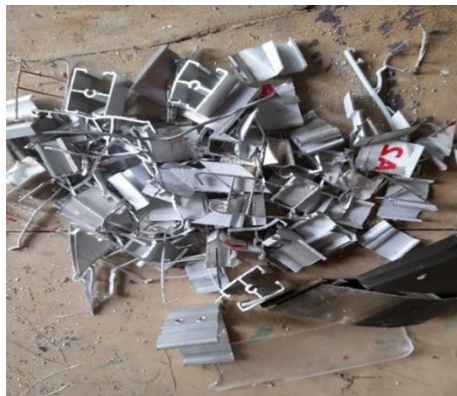
Figure 3.8 Waste Aluminium Recovered from Aluminium Door Frame Producers
