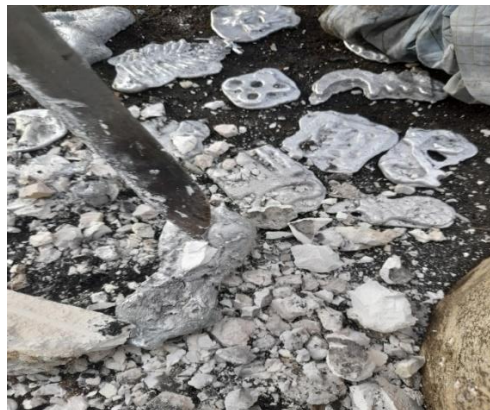
Figure 3.50 Breaking the Mould
