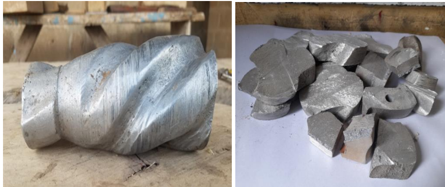
Figure 3.7(b) Waste Aluminium Recovered from Fufu Pounding Machine
