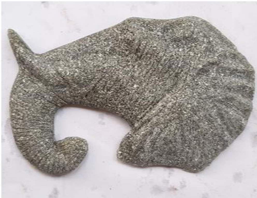
Figure 4.1 Final Cast of Head of an Elephant from Solid Waste Aluminium Chips
