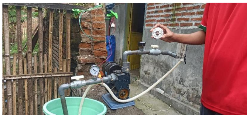
**Gambar 6.** Uji coba impeller
